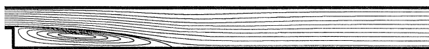
Figure 3. Steady streamline portrait for flow down a backward step. The Reynolds number is 250 and the channel length is 20. A parabolic laminar profile at the inlet and Dirichlet boundary condition at the outlet are used. The solution is obtained using the finite-difference code developed by Kim & Moin (1985).
